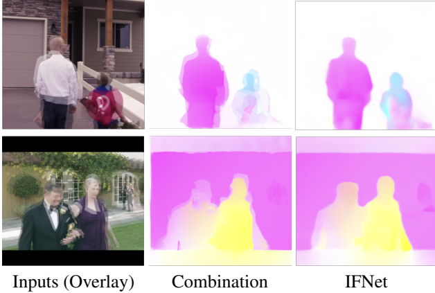
Figure 5: Visual comparison between linearly combined bi-directional flows generated by a pre-trained LiteFlowNet [11] and the intermediate flow approximated by IFNet. IFNet produces clear motion boundaries.
