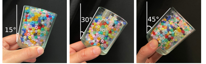
Fig. 4: Fill levels used in open-top container transport experiments. As we use beads (instead of liquids) for safety and ease of cleanup, we fill containers to just before spilling.
