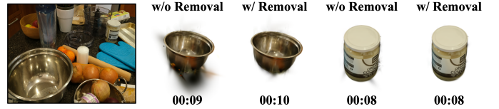
Fig. 10. The effect of the ambiguous Gaussians removal strategy for SA3D-GS. Experiments are conducted on 360-counter [6]. Corresponding segmentation time cost is labelled below each segmentation result. This strategy can eliminate ambiguous Gaussians at the border of the segmented target within one second.
