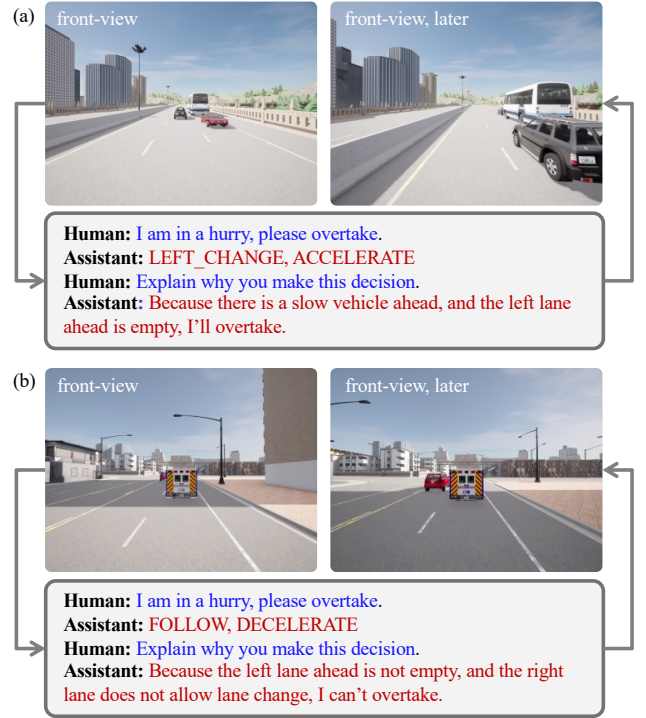
Fig. 5 Visualization of human interaction with DriveMLM, featuring examples of (a) a successful overtake and (b) a failed overtake due to unreasonable demands rejected by DriveMLM. In each example, the left image captures the moment of giving instructions, while the right image represents a subsequent stage of instruction execution.
