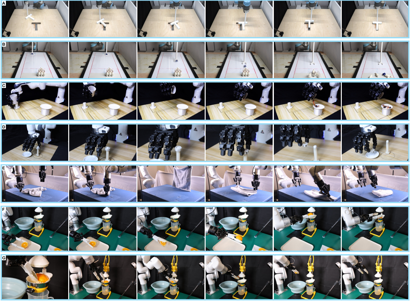
Figure 3. Illustrations from rollouts on seven real-world tasks. Each row shows one task, and columns are time-ordered frames (left→right) subsampled from a single trajectory. From top to bottom: (a) Dynamic Push-T, (b) Agile bowling, (c) Pouring, (d) Dynamic Unscrewing, (e) Soft-towel Folding, (f) Orange Juicing – Placing, (f) Orange Juicing – Removal. The suite spans fluids or particles, tool-using, deformable objects manipulation, dynamic non-prehensile manipulation, and precise insertion, highlighting the diversity and dynamics of our benchmark.
