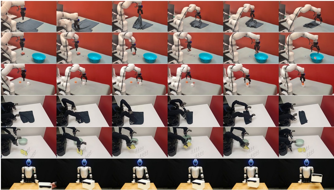
Fig. 3: VLA manipulation trajectories. We showcase rollouts of \pi_{0.5} across 3 morphologies on 5 diverse tasks, shown at 0%, 20%, 40%, 60%, 80%, and 100% of task completion.
