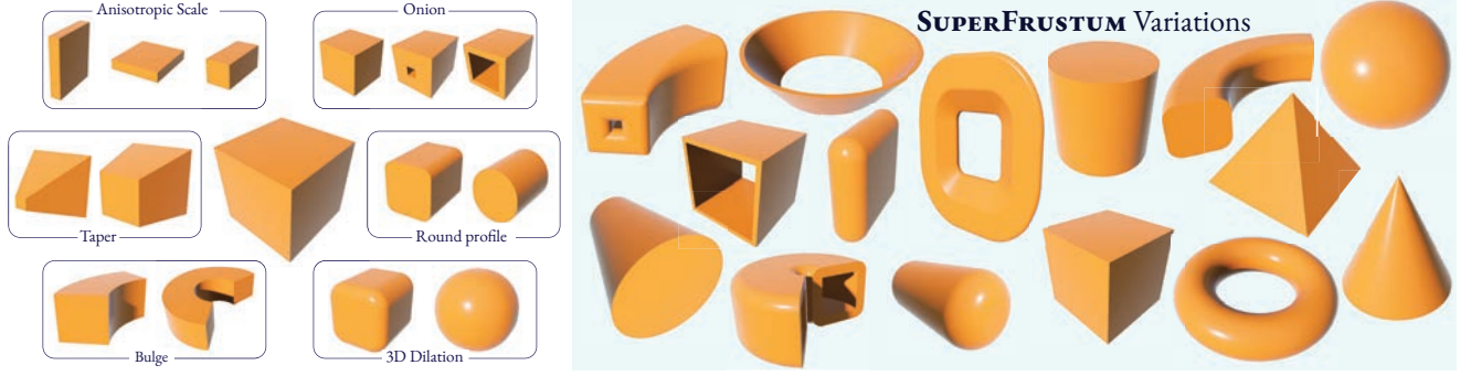
Figure 2. SuperFrustum—An Expressive, Compact & Differentiable Primitive. SuperFrustum is a unified analytic SDF primitive with only 8 parameters controlling dilation, taper, bulge, onion-like hollowing, profile roundness, and axial scaling. Its SDF is C^0 -continuous and fully differentiable (almost everywhere) with respect to all parameters, enabling robust inverse modeling and gradient-based optimization. As shown on the right, these parameters allow a single formulation to morph smoothly across common solids—cuboids, cylinders, cones, spheres, and toroidal variants—and to produce more complex shapes such as bent, hollow, or smoothly capped forms.
