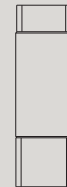
D2 (ADT7278) Fit 7/8 Square Tube Exp. 0.852 - 0.927 13/32 Square Top Round Rubber 3/4 Square Base
