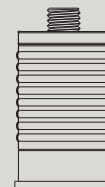
S6 (ASP7615) Fit 1-1/2 Round Tube Exp. 1.426 - 1.589 S.S. Knurled Nut Round Rubber and Plastic Bushing S.S. Base Washer
