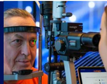
**Modulight ML7710** is a **multi-indication** and multichannel laser platform designed for demanding medical environments. Engineered for both clinical and research applications, ML7710's cloud-connectivity and intuitive user interface make it suitable for various medical applications, ranging from **photoimmunotherapy (PIT)**, **photodynamic therapy (PDT)** to **fluorescence imaging** and **photothermal therapy**.
