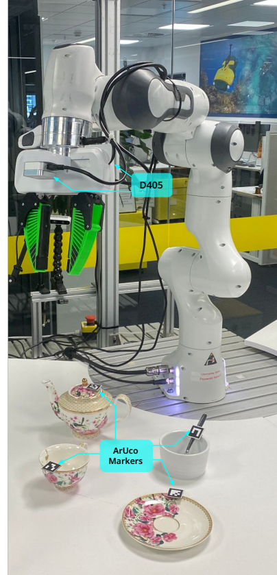
Figure 13: Experimental Setup. Franka Panda manipulator robot equipped with 2 D405 Realsense cameras. Objects with ArUco markers for affordance-centric frame detection and tracking.
