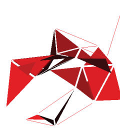
Figure 10–6 3D Delaunay triangulation with non-zero alpha.
