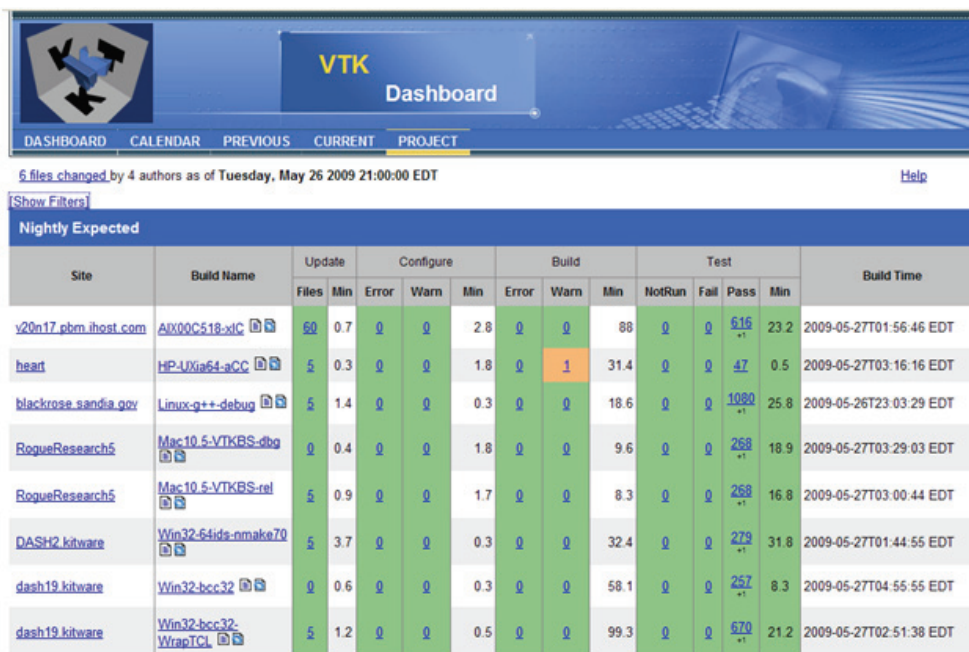
Figure 14–1 CDash regression testing dashboard. Tests are submitted from client sites around the world. The dashboard summarizes the results of hundreds of tests, and makes those results available as hyperlinked Web pages that is publicly viewable.
