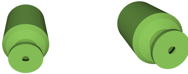
Figure 4-4 The effects of applying rotation in different order. On the left, first an x rotation followed by a y rotation; on the right, first a y rotation followed by an x rotation.
