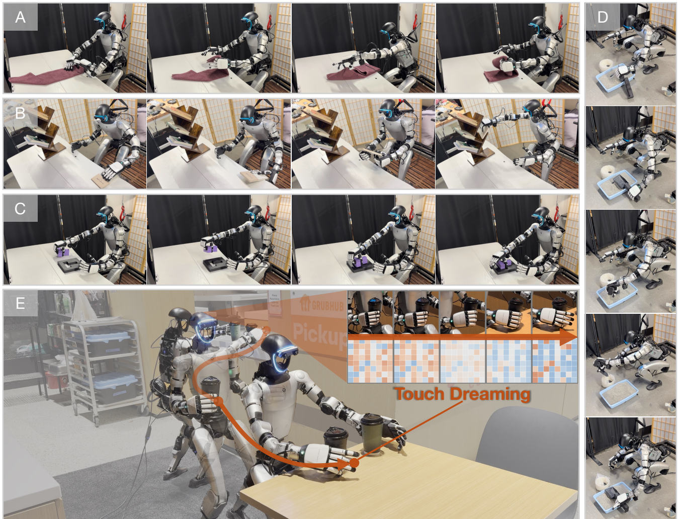
Fig. 1: Our system enables versatile , contact-rich , and dexterous humanoid manipulation. A : long-horizon, multi-stage manipulation of deformable objects (towel folding). B : mixed prehensile and non-prehensile manipulation for thin-profile rigid objects with limited grasp affordance (book organization). C : tight-tolerance insertion with a clearance of 3.5 mm, requiring high precision and reactive adaptation (Insert-T). D : dexterous, tool-mediated contact under low-profile constraints (cat litter scooping). E : bimanual object fetch and loco-manipulation, requiring stable whole-body transport while keeping objects balanced (tea serving); the embedded panel visualizes touch dreaming by showing the dreamed tactile latent of the right middle finger as a normalized heatmap that changes with finger-object contact.
