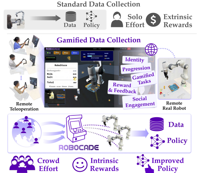
Fig. 1: We develop RoboCade , a platform that gamifies the collection of robot demonstration datasets. In standard data collection approaches ( top ), hired operators or researchers collect demonstrations using in-person teleoperation, which requires access to a robot and can be tedious and time-consuming. RoboCade ( bottom ) is a remote data collection platform that integrates gamification into both system and task design, making robot data collection more engaging and accessible to a broader set of users.
