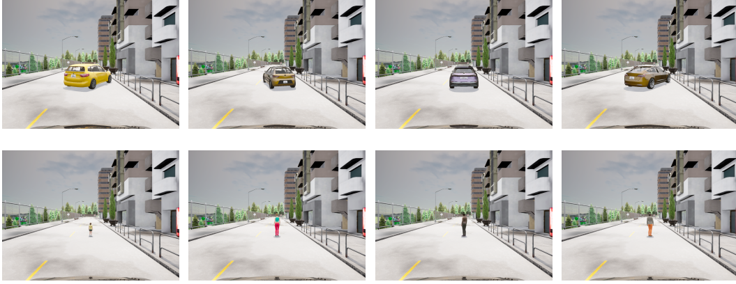
Figure 9: Physical semantic perturbations and transformations of vehicles and pedestrians. For vehicles, we consider different types, colors, and rotations. For pedestrians, we consider different body shapes, skin colors, and rotations.
