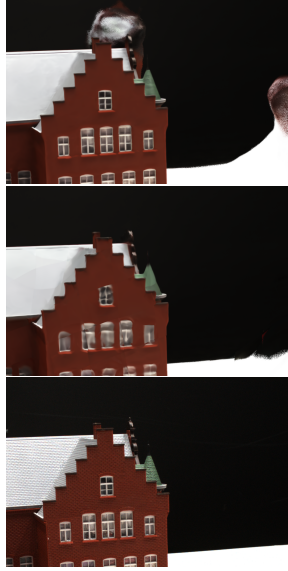
Figure 6. Rendering artifacts in the NeuS representation (top), KiloNeuS improvement (center), and ground-truth image (bottom).
