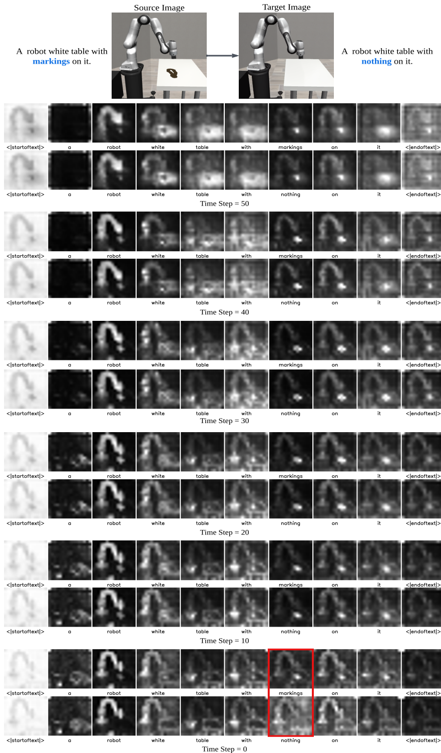
Figure 8: Attention visualization of Prompt-to-Prompt. The visualization of cross-attention maps at diffusion step t = 50, 40, \dots, 0 , with the cross-attention maps generated by the source diffusion process (upper row) and the target diffusion process (bottom row). The first 40 steps keep the original structure of the source image, and the required editing is performed during the last 10 diffusion steps, as indicated by the red box.
