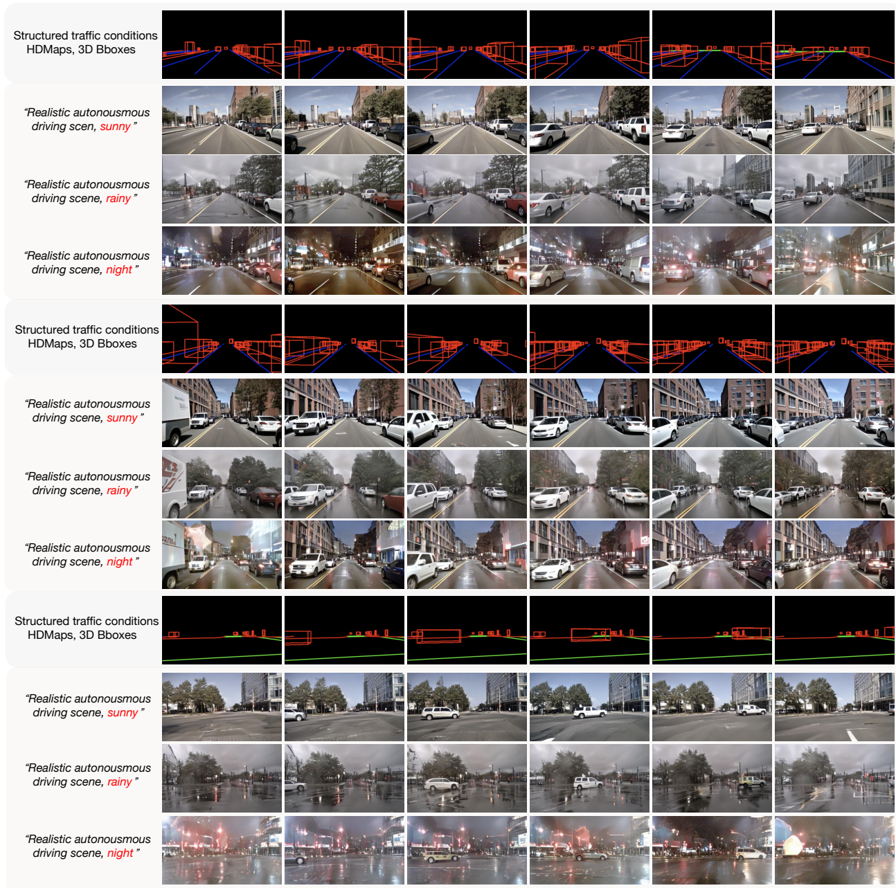
Figure 9. Driving video generation with structured traffic conditions (HDMaps and 3D boxes), where text prompts are utilized to adjust driving scenario style (e.g., weather and time of the day).
