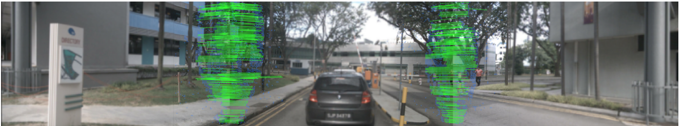
Figure 22. Illustration of keypoint matching in KPM calculation. The blue points are the image keypoints in the overlapping regions on the left/right side of the image. The green lines are the matched keypoints between the current view and its two adjacent views using the LoFTR [51] matching algorithm.
