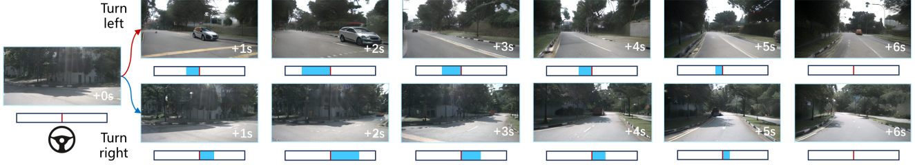
Figure 14. Diverse turning behaviors. Utilizing an identical initial frame, we provide our model with sequences of positive steering angles (indicating a left turn) and negative values (indicating a right turn). The figure demonstrates the model’s proficiency in generating consistent street views for both turning behaviors. Each frame is accompanied by a blue bar, indicating the corresponding steering angle in degrees. A longer bar correlates with a more substantial steering angle. For clarity, only the front view is shown.
