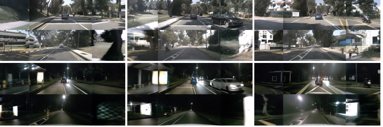
Figure 12. Lighting change generation. The top row displays daytime scenes. The bottom row shows the same layouts rendered as nighttime scenes, demonstrating conditional generation capabilities.
