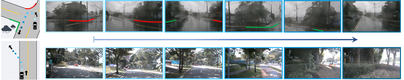
Figure 7. Counterfactual events generation. Top: turning around at a T-shape intersection on a rainy day. Note that our training set does not contain any turning-around samples. Bottom: running over a non-drivable area.
