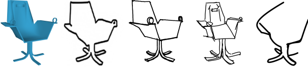
Figure 5. From left to right: 3D shape; an edgmap of a 2D render of the shape; corresponding sketches from the ProSketch3D [91] and AmateurSketch3D [61] datasets; an abstract CLIPasso [70] sketch of the shape.
