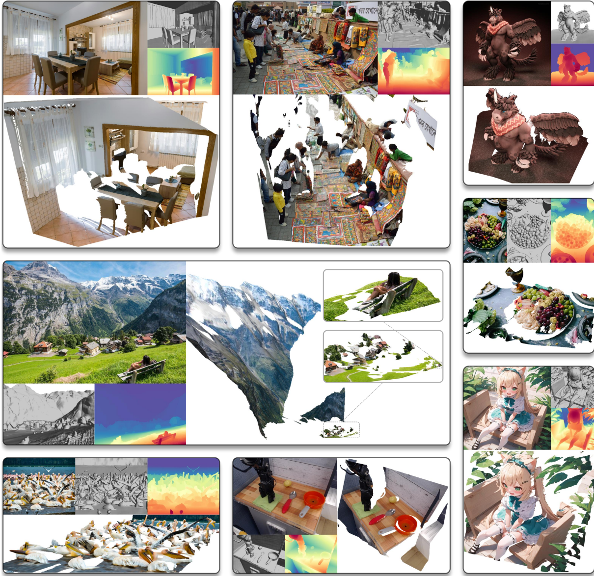
Figure 1. Given any image, our method reconstructs an affine-invariant 3D point map of the scene and can also produce a depth map and the camera focal length. The model yields high-quality shapes and generalizes well to open-domain images. ( Best viewed with zoom )
