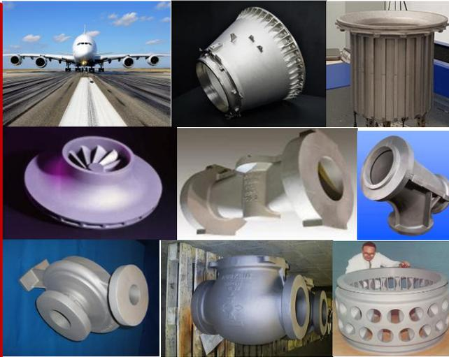
**With 40 years of experience, SETTAS provides in-house engineering and production, co-developing complex parts. SETTAS casts large titanium components up to 2600 mm in diameter using sand casting (as an alternative to forged components or large welded assemblies).**
