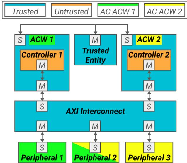
Figure 3: Block diagram of the Multi ACW design
