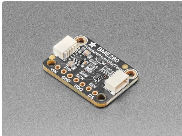
[Adafruit BME280 I2C or SPI Temperature Humidity Pressure Sensor](https://www.adafruit.com/product/2652)
