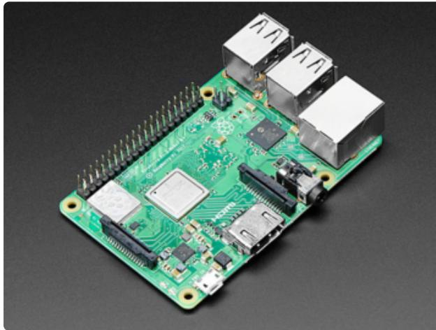
1 x I2C port with **busio** (but clock stretching is not supported in hardware, so you must set the I2C bus speed to 10KHz to 'fix it')
