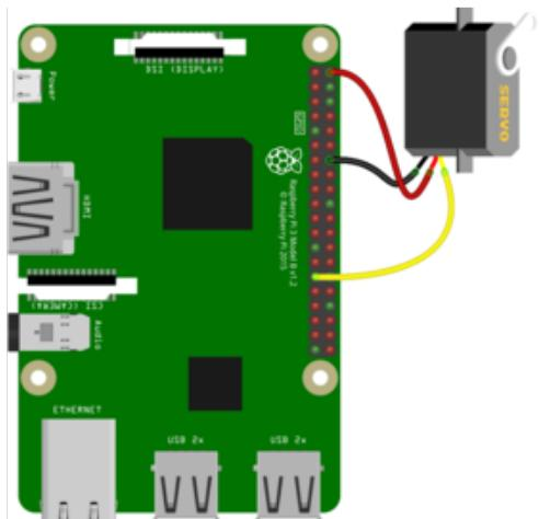
Servo power (red wire) to Raspberry Pi 5V
