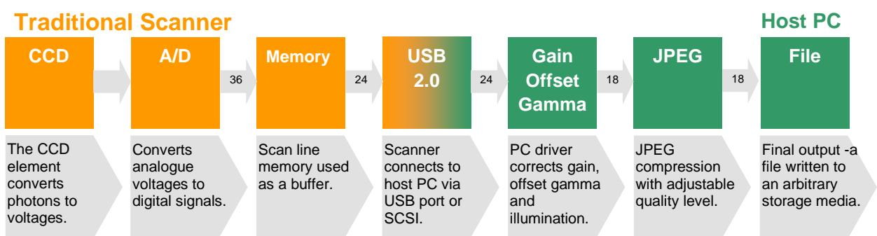
In a Scan2Net® scanner, all corrections as well as gamma are performed inside the scanner at the full resolution of the camera subsystem, typically 36bits. Only the clean, compressed file is send to the PC via the network, not only reducing traffic but preserving much more resolution.
