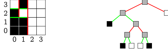
Figure 13.3 Image and corresponding k -d tree
