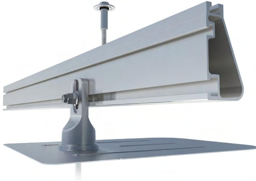
The IronRidge Flush Mount Systems are rail-based systems for mounting solar modules on pitched roofs. The systems utilize IronRidge XR Rails® or Aire® Rails with a variety of roof attachments to support extreme wind and snow loads. The entire system uses only aluminum and stainless steel components to ensure complete corrosion resistance.
