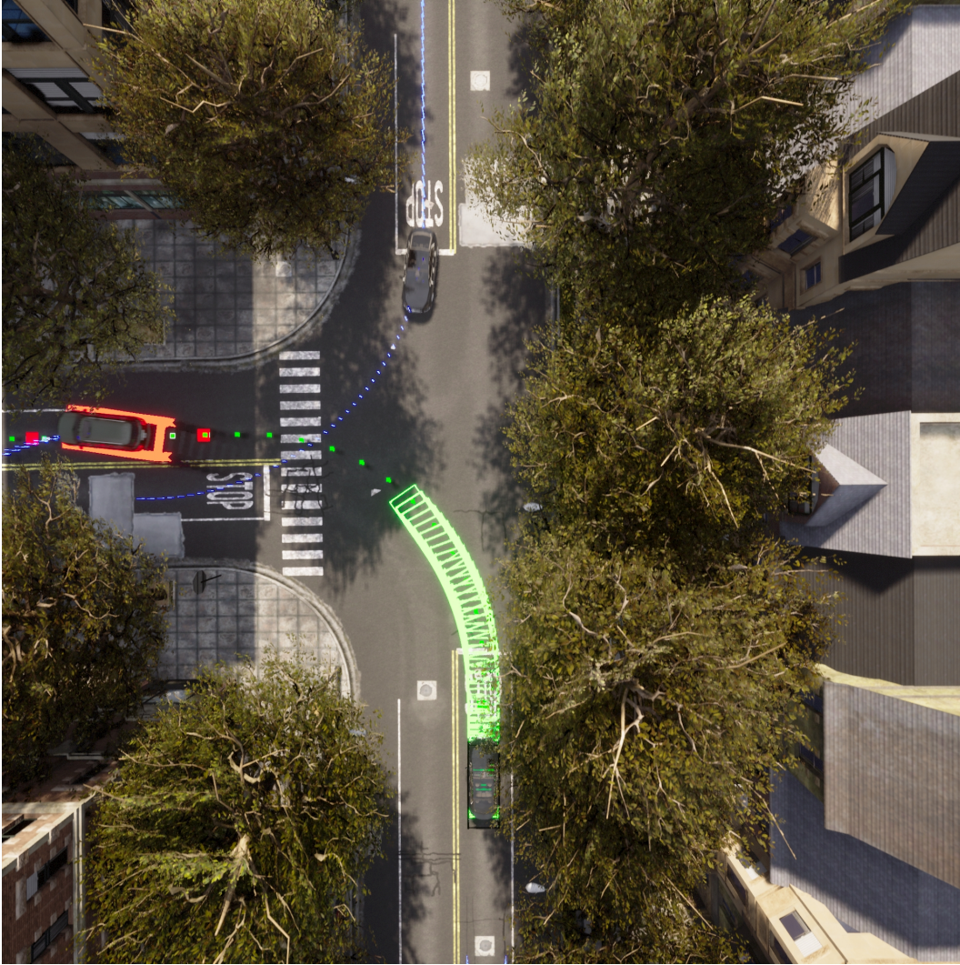
Figure 4.9: Unprotected left turn with competing Flow. Both front and rear collisions are possible if the model fails to find a suitable gap in time.
