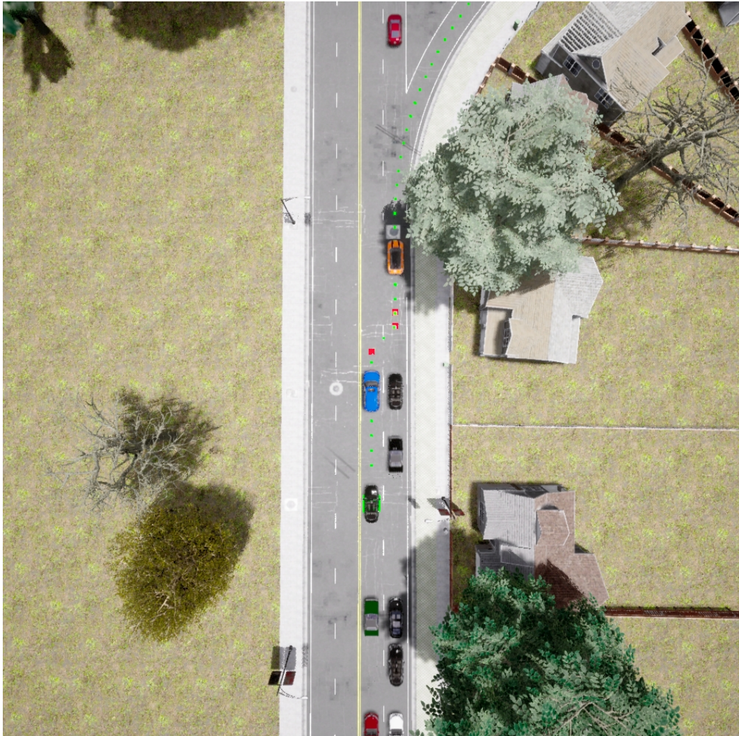
Figure 1.1: Example of a limited navigation system in CARLA. The driving model sees only the red points, the output of the navigation system. The lane change is abrupt, and the fork offers ambiguous visual cues about whether to stay on the main road or take the exit. Attempting the lane change too early or too late often results in an out-of-lane violation or collisions. Even worse, missing the exit would immediately terminate the evaluation. This highlights a limitation of current long-route evaluation protocols, where overly strict success criteria penalize reasonable driving behavior, which mostly come from insufficient navigation conditioning.
