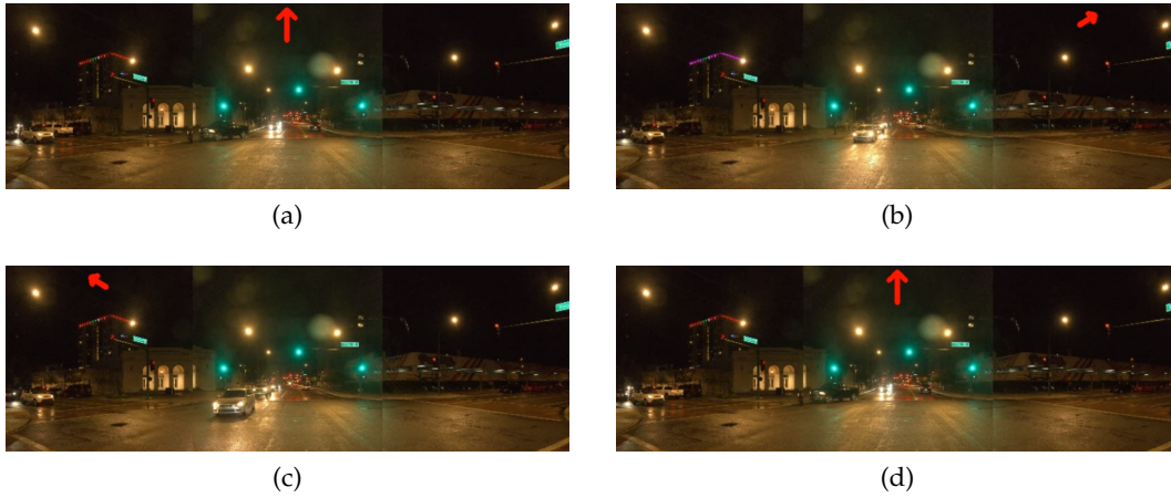
Figure 3.4: Temporal inconsistency in automatically generated navigation commands. Red arrows visualize the discrete command at each timestamp (straight, left, or right). All four frames show the same intersection scenario captured at consecutive timestamps, yet the commands flicker between different directions, exposing the lack of temporal coherence in the navigation signal.
