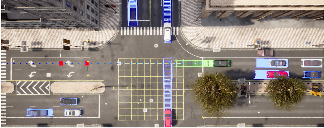
Figure 4.8: Defective traffic lights. The ego has to find gaps in slow but continuous cross traffic to proceed through the intersection.
