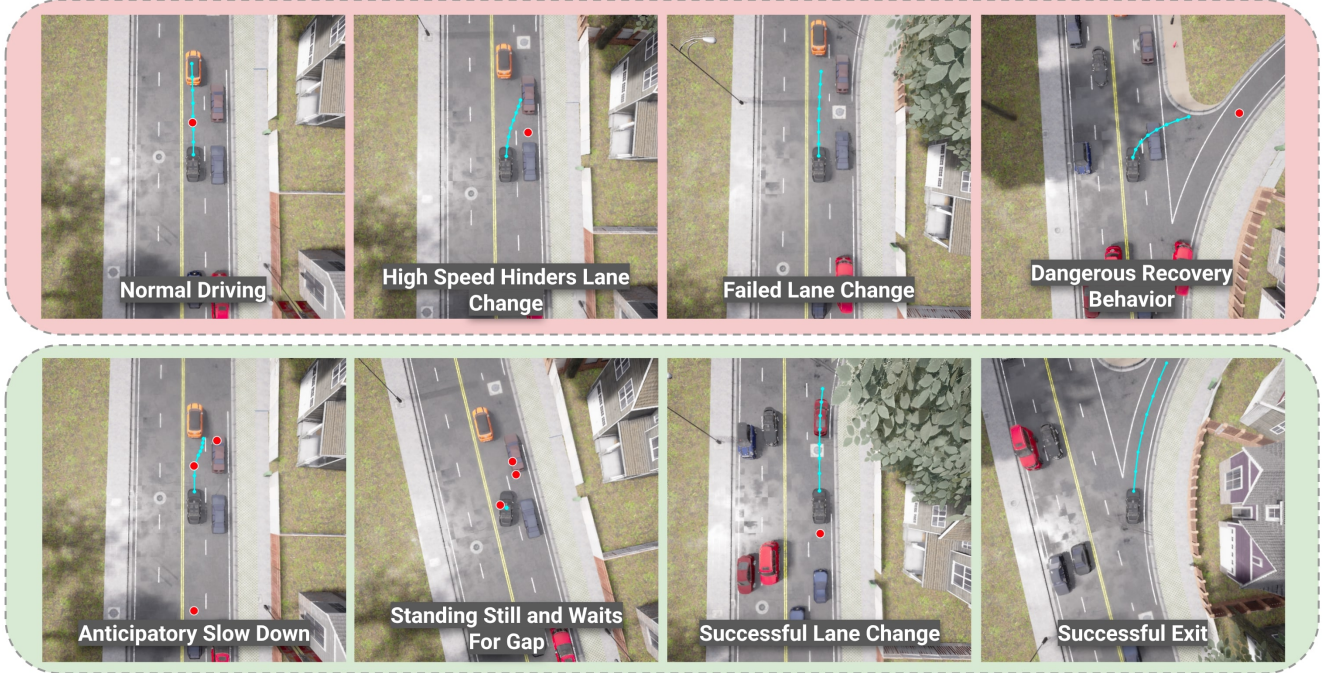
Figure 1. Top. Limited intent conditioning results in ambiguous behavior and makes TFv5 miss the exit. Bottom. TFv6 resolves these ambiguities through improved intent conditioning, enabling reliable lane-change execution and safer interaction with surrounding traffic.
