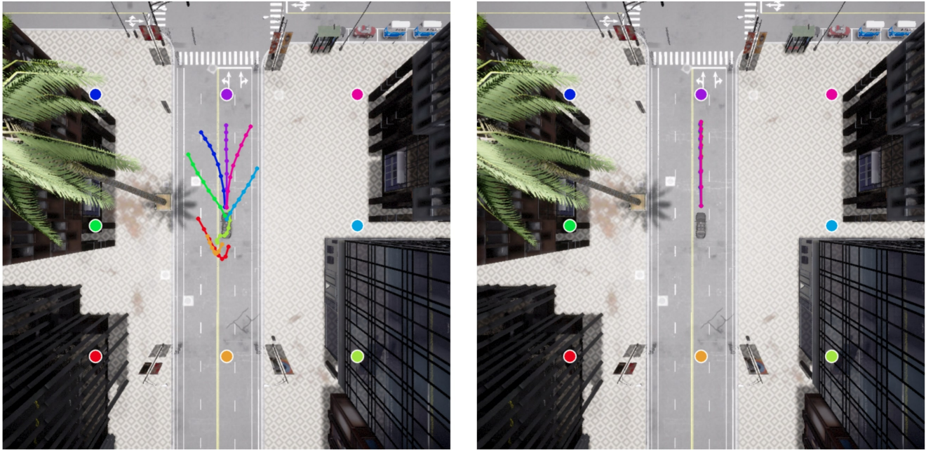
Figure 4. Effect of the current target point on the planning output before ( left ) and after ( right ) intent alignment. In the pre-alignment model, the predicted trajectory follows the target point almost verbatim. After intent alignment, the learner interprets target points more robustly and produces a consistent, lane-aligned plan. While this reduces the tendency to overreact to small variations in target-point placement, it also removes the “recovering” behavior that occasionally helped the model correct itself on long-route evaluations.
