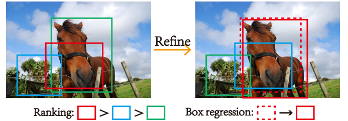
Figure 1: Overview of object proposal refinement. The left image shows the original proposals, and the right image shows the results after refinement. We first re-rank the proposals by computing new objectness scores, after which a box regression procedure is applied to each proposal box for accurate location.
