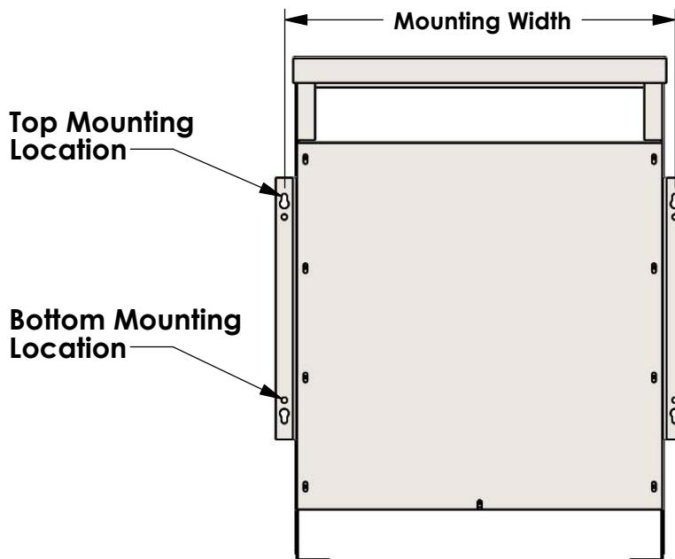
To mount the unit on the wall, first install two bolts (not included) on the desired wall at the correct mounting width apart and at your desired height (Minimum bolt size is 5/16" and of a suitable length and type for the intended mounting surface). Hang the transformer like a picture from these bolts at the top mounting locations. Next install two bolts with washers at the bottom mounting locations. Then (ONE AT A TIME) remove the top bolts to add a washer and re-install them.
