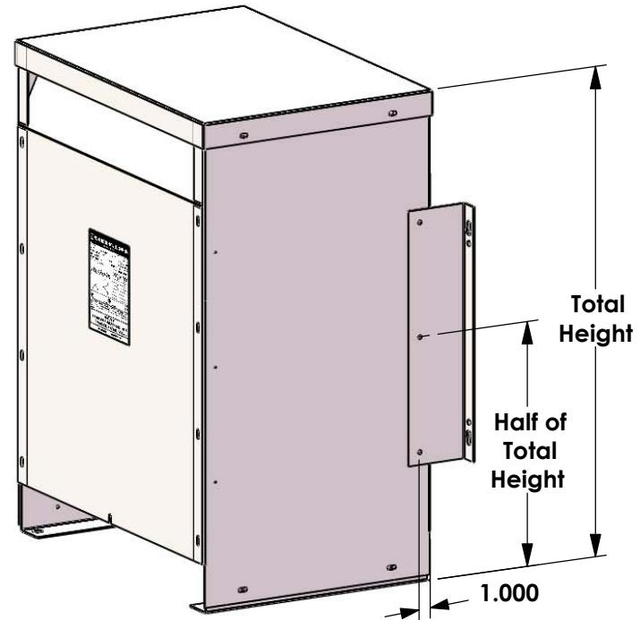
To attach wall mount brackets, put one of the included 5/16 x 1" self-drilling/tapping screws through the center hole of the wall mount bracket and through the case. It should be 1" from the rear of the case to the hole and at the centerline of the cases vertical height. Then add the other 2 adjacent screws. Repeat for other side.
