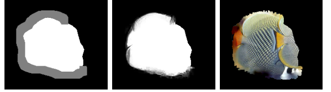
Figure 6: Alpha matting. (Left to right) For the second fish on the last row in Figure 1 the extracted trimap, alpha value, and foreground color, respectively.
