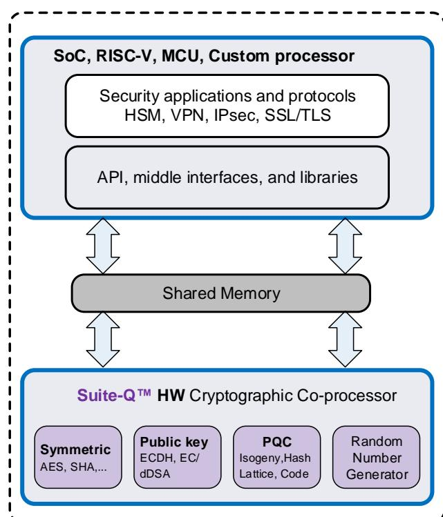
**Suite-Q™ HW** offloads the following symmetric and asymmetric cryptographic operations and makes the executions more efficient.
