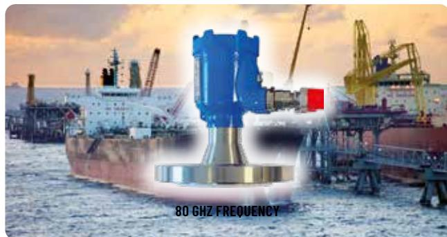
Scanjet high frequency pulse radar, ScanRad, is a high performance instrument for measurement of level/ullage in tanks. The compact design ensures easy and flexible installation. Purpose developed software enables the user to filter any echoes from obstacles in the tank to ensure accurate reading.
