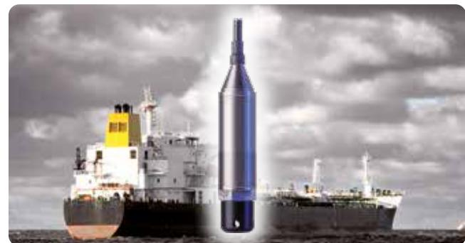
Custom-made high-quality pressure transmitters measure absolute or gauge pressure depending upon the application. Transmitter construction is fully laser welded and internally encapsulated to ensure complete sealing. Materials of construction are SS316L, Titanium, Hastelloy to suit all shipboard fluid. All are rated IP68 and suitable for permanent submersed operation. Transmitters are Marine Type approved and Certified Intrinsically Safe for hazardous Area applications.
