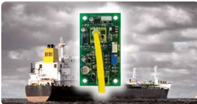
The SML-1000 electro pneumatic system offers continuous measurement providing DC 4-20 mA or digital Modbus outputs to central display units, to Integrated Alarm Monitoring System and to Loading Computer. The largest systems delivered is composed of 20 cabinets in different fire zones, which monitor more than 250 measuring points.
