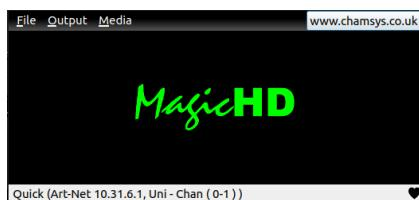
The main window shows status bar shows the network configuration, with DMX health on the right. A black heartbeat means DMX data is being received. A green heartbeat means the values are changing. ``No DMX" flashes when no data is being received.
