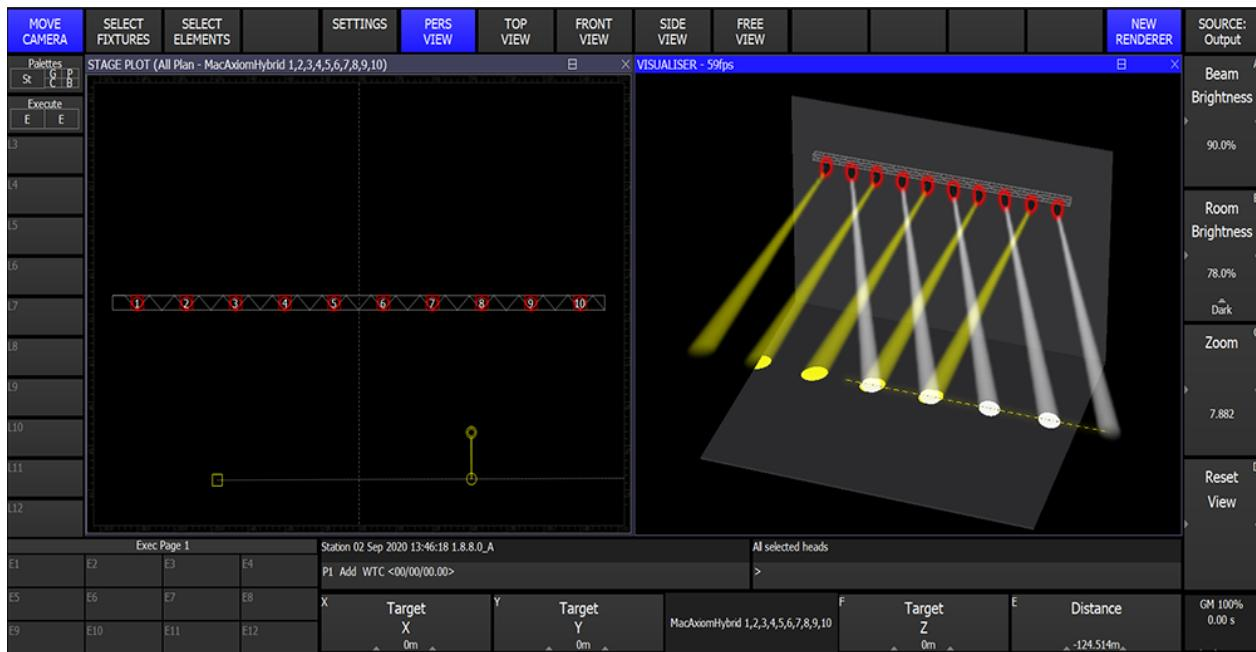
The 'Base Position' is the starting position for the heads before they are panned around to focus on the point. If the head has to pan more than 90° from the base position it will 'flip' the head over. The default base position is directly downstage. If the lights flip while they are moving between positions a different base position may be required.
