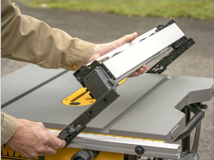
Step 2. Lift the DeWalt Rip Fence off the table and place on an flat tabletop.
