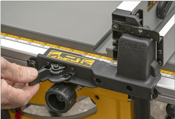
Step 1. Unlock the fence levers located on the front and back of the DeWalt Fence Assembly .
