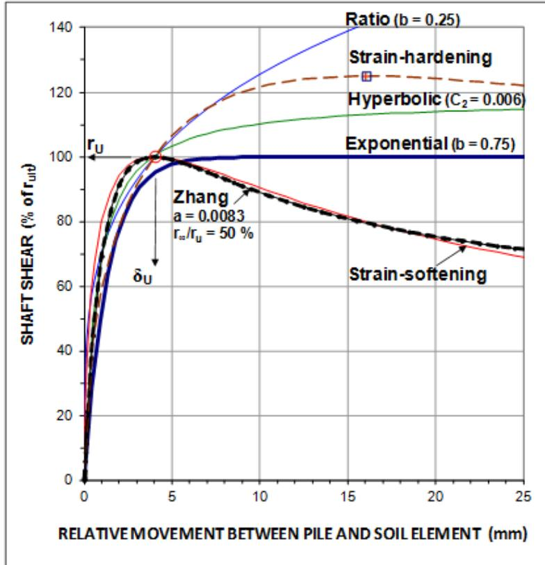
**Fig. 1. Six t-z or q-z functions with a common 100% ultimate resistance value for a movement of 4 mm. The strain-hardening and strain-softening curves are calculated according to the Hansen 80-% method**
