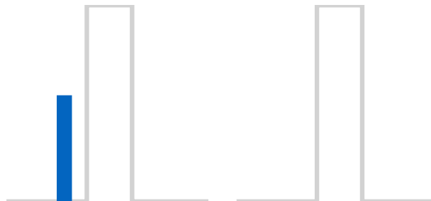
Figure 20-14 Camera-and-LED timing diagrams showing LED synchronization failures: (left) LEDs flash outside the camera exposure period; (right) LEDs do not flash at all
