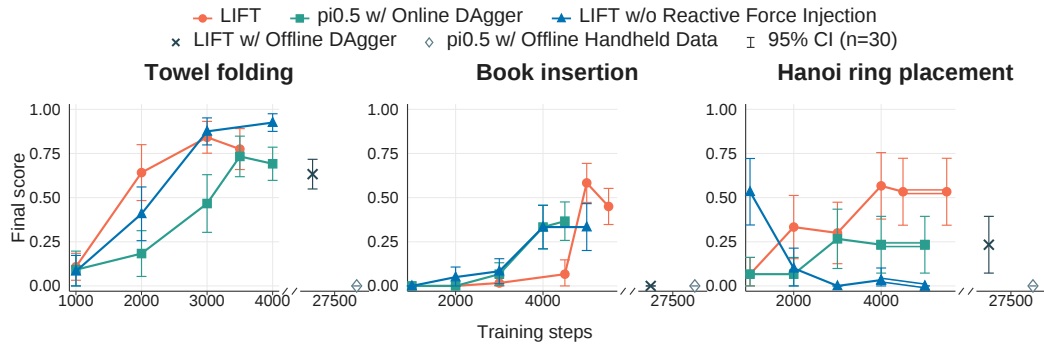
Figure 5: Learning curves on three tasks as training steps increase. Force-enabled post-training improves adaptation over vision-only online DAGger.
