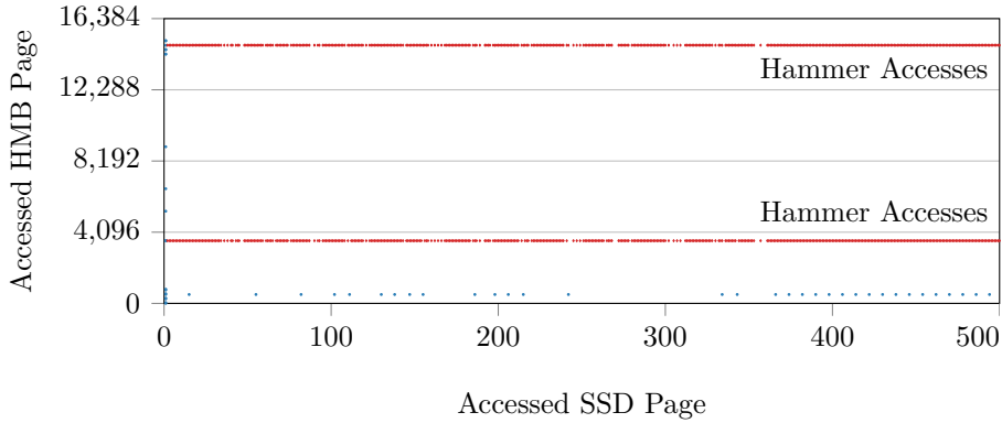
Figure 8.6.: The hammer accesses from the Samsung 980. The first access to the SSD causes many HMB accesses. Then it takes 360 accesses for the SSD to “settle in”. Afterward, every single access to the SSD, causes the SSD to access pages around index 3 606 and 14 854 of the HMB.
