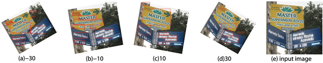
Fig. 3 Find candidate text regions by first rotating the image and then applying SWT [1]. (a)–(d) are text detection results with the image being rotated at -30^\circ , -10^\circ , +10^\circ , and +30^\circ , respectively. (e) is the original input image for text detection. When rotated by +10^\circ , no text is detected
