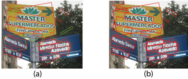
Fig. 4 Remove inconsistent candidate text regions. (a) shows all candidate text regions detected in the previous step, where the green regions are the inconsistent ones. (b) is the remaining candidate text regions after removing inconsistent text regions
