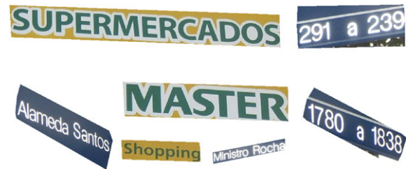
Fig. 8 Convex hulls of different groups of re-detected text areas. We first find groups of rectangles whose pairwise overlapping ratio is greater than 0.7. After removing inconsistent rectangles by principal directions, we calculate the convex hull of each rectangle group and segment the hulls out of the original image
