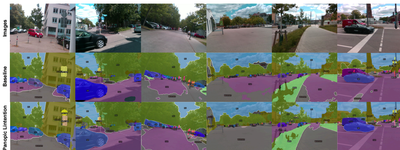
Fig. 4: Comparison with the baseline Panoptic FPN on real-world images. Raw RGB image, baseline results, and Panoptic Lintention results are organized from top to bottom. Best viewed in color.
