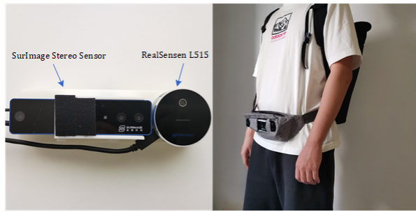
Fig. 1. RealSense Camera L515 is integrated on the belt and connected with the processor NVIDIA Jetson AGX. As a multi-sensor system, SurImage Stereo Camera complements the RealSense in various conditions.
