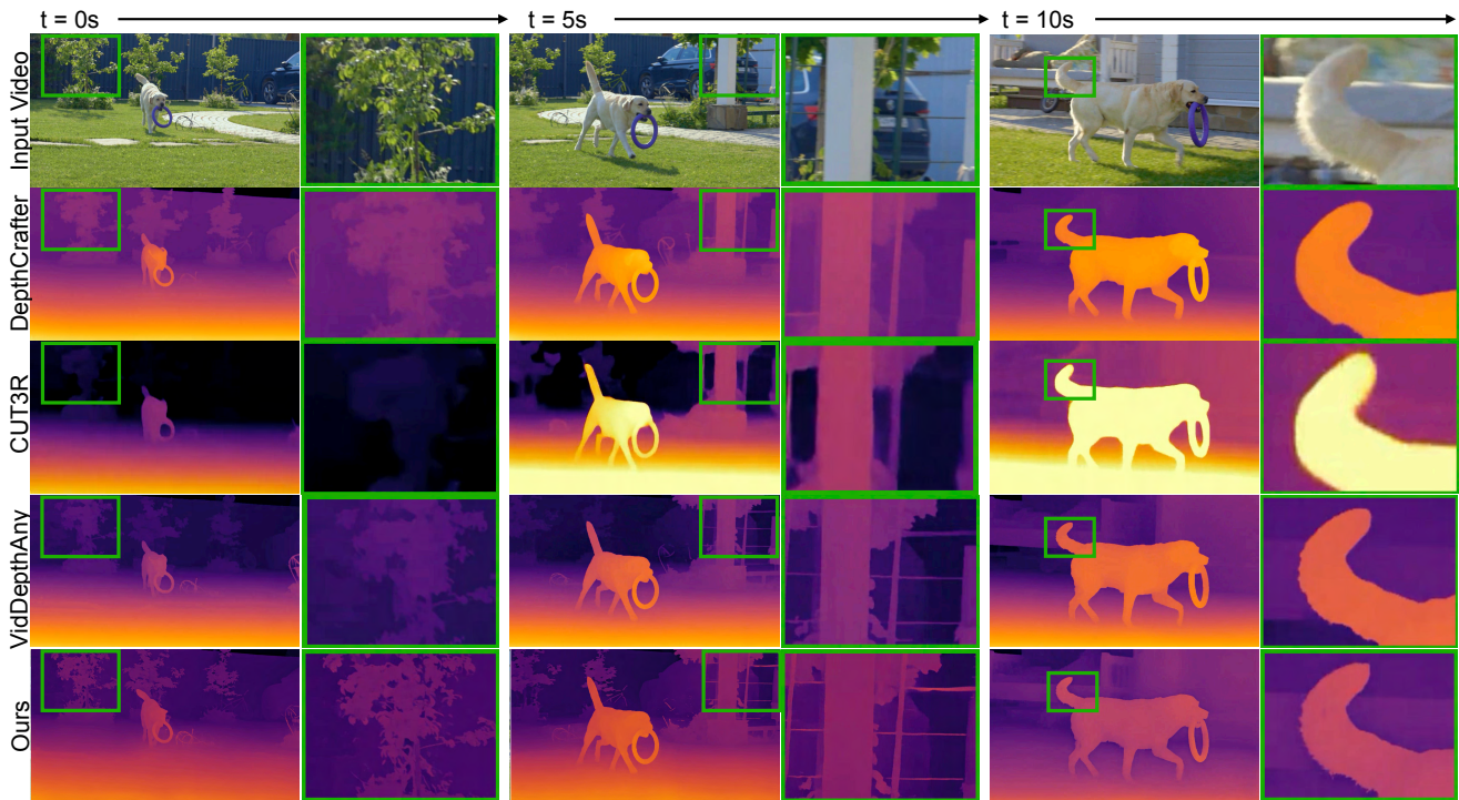
Figure 1. We present FlashDepth, a video depth estimation model that processes high-resolution streaming videos in real-time. Given an in-the-wild video shown above (left column: original input and output; right column: zoomed-in), our method processes it in a streaming fashion at 2044 \times 1148 resolution at 24 FPS . In contrast, the state-of-the-art video depth model, DepthCrafter [25], runs at 2.1 FPS at 1024 \times 576 resolution and requires optimizing 110 images at once. Concurrent works like CUT3R [56] supports streaming inputs ( 512 \times 288 at 14 FPS) but produces blurry depth; Video Depth Anything (VidDepthAny) [8] runs at 24 FPS at 924 \times 518 resolution but requires optimizing 32 images at once. Our predicted depth maps are noticeably sharper than all baselines, capturing thin structures such as tree leaves and fur. Zoom in for best viewing results.
