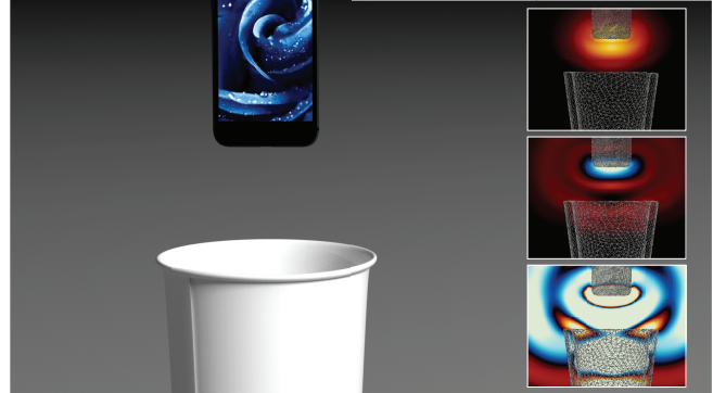
Fig. 14. Area source 3D re-recording shader. For a directional sound source, the user inputs a surface patch they want to apply the source on. We then directly specify the Neumann boundary condition. In this example, we attached two rectangular patches at the bottom of the phone and play the familiar “marimba” ringtone.
