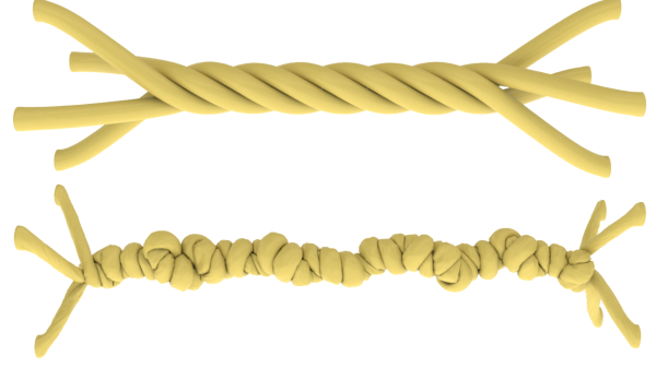
Fig. 4. Extreme stress test: rod twist for 100s. We simulate the twisting of a bundle of thin volumetric rod models at both ends for 100s. IPC efficiently captures the increasingly conforming contact and expected buckling while maintaining an intersection- and inversion-free simulation throughout. Top: at 5.5s, before buckling. Bottom: at 73.6s, after significant repeated buckling is resolved.
