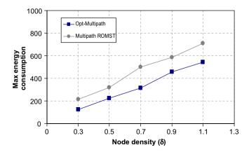
Fig. 5. Maximum energy consumption vs. node density under MP routing.
