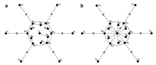
Fig. 3. An example that shows the node degree in OMST can reach 12. The number on each link is the length of that link. Note that  $d \gg d'$ . (a) MST of the network. (b) OMST of the network.
