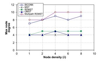
Fig. 7. Maximum node degree vs. node density.
