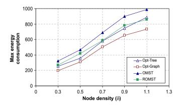
Fig. 4. Maximum energy consumption vs. node density under SP routing.
