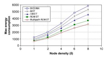
Fig. 6. Maximum energy consumption vs. node density.
