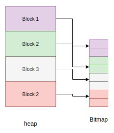
The bitmap tracks whether a block is "free" or "in use" and use two bits to track this state for each block.
