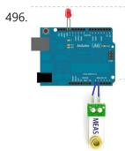
How to Build a Vibration Detector Circuit In this project, we will go over how to build a vibration detector circuit. This is a circuit which can detect and measure flex, touch, vibration, and shock. The sensor we will use to detect these movements is a piezo vibration sensor from Measurement Specialists (MEAS). The..... Listed under: Sensor – Transducer – Detector Projects
