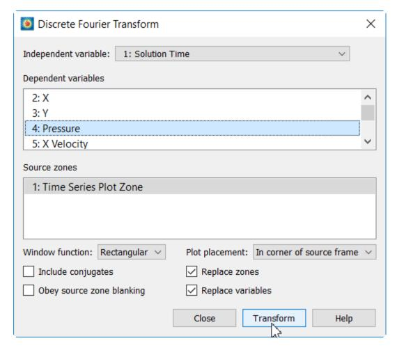
In this dialog, choose Pressure as the dependent variable and make sure the Time Series Plot Zone is selected as the source zone. Using the **Plot Placement** drop-down menu, choose to tile the new frame with existing frames. Leave everything else the same. Click **Transform** to perform the Fourier transform.
