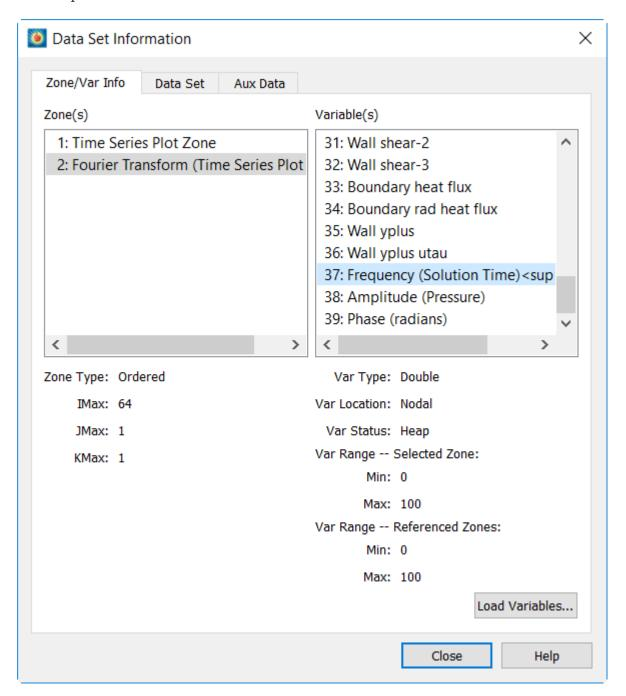
As you can see, Tecplot 360 has created a new Fourier Transform zone based on the Time Series Plot and added three new variables starting with variable 37. (The other zone and the first 36 variables were created when we generated the time series plot.)
