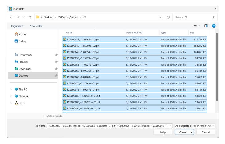
Navigate to your Tecplot 360 Getting Started Bundle folder then the Internal Combustion Engine (ICE) folder. Select all of the .plt files and select Open. The data files are opened and a 3D plot of the Combustion Engine appears in the Tecplot 360 workspace, as shown here:
