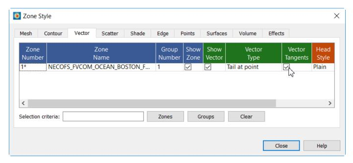
Select the Vector tab and then select the checkbox under "Vector Tangents". This will ensure that the vectors will be displayed tangential to the surface. Close the Zone Style dialog.
