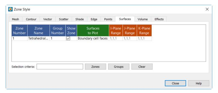
Navigating to the Surfaces tab, you'll see that the Surfaces to Plot heading has changed to **Boundary** cell faces which allows us to see the contour of surfaces of exposed boundary cells.
