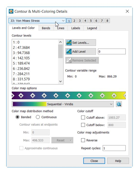
Next, select the **Set Levels...** button and change the minimum level to be 0, maximum level to be 900, and the number of levels to be 21. The resulting **Enter Contour Levels** dialog should look like the picture below. Select **OK** and Close the **Contour & Multi-Coloring Details** dialog for now.
