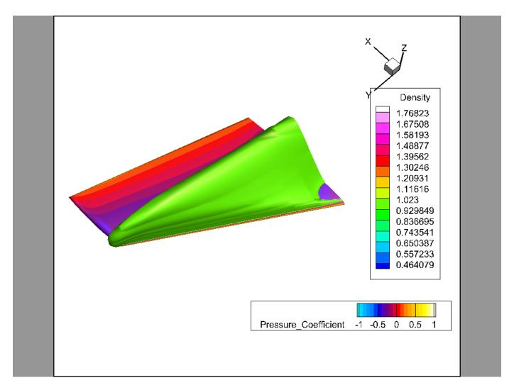
This iso-surface shows us where the air is moving at Mach 1 around the wing. Try adjusting the Value 1 field using the arrows next to the numeric entry field and watch the plot change in response.
