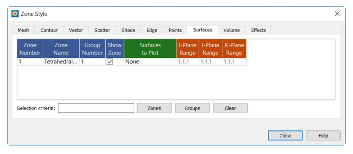
For performance reasons, the default option for **Surfaces to Plot** is set to "none" on volume zones. When you have a volume zone where you'd like to see the surface data then change this option. Note that if surface zones are in the dataset, they would be shown in the Zone Style dialog as "N/A".
