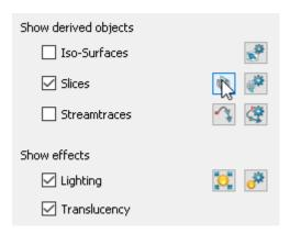
A slice appears through the volume zone but may be hidden by surfaces. To be able to see the slice through the middle of our engine we must turn on Translucency in the Plot Sidebar as well.
