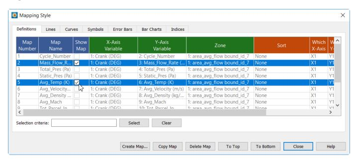
Notice how the plot automatically merges both lines to one Y Axis. The min/max values of Mass\_Flow\_Rate and Avg\_Temp are very different, so putting one of the mappings in a second Y axis will help.
