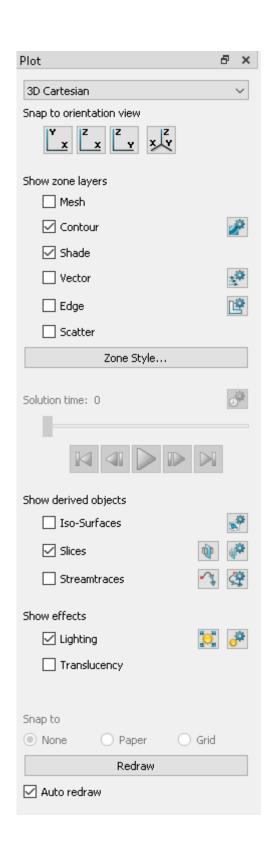
To add a slice, toggle on the Slices checkbox in the Plot sidebar. A slice appears through the volume zone.
