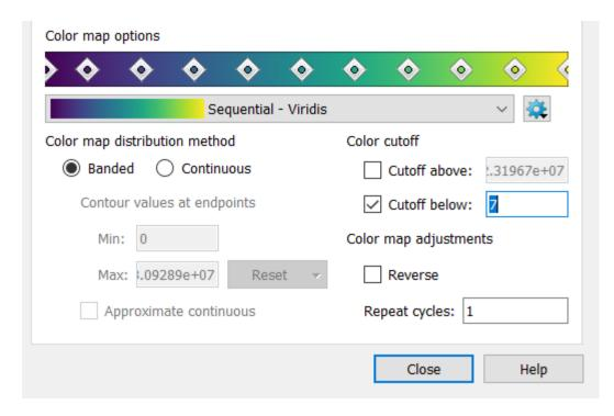
This makes our vortices stand out by eliminating all contouring below 7. You might experiment with slightly lower and higher values to see more or less. Now we must remove the legend as it is overlapping a region of interest on our plot.
