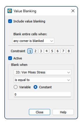
The resulting plot isolates the connecting rod because the Von Mises stress contour values are equal to zero on the crankshaft and cylinder. Though the parts still exist in the data set, they do not give helpful information. In the Value Blanking dialog, multiple constraints can be enabled at once to confine the plot view to very specific areas. For this situation, only one constraint was needed.
