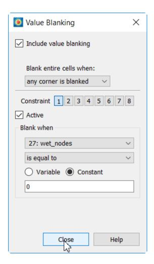
Then turn on the "Include value blanking" checkbox. This will tell the plot that we want to blank something. Change the Blank when fields to be when "wet\_nodes", "is equal to", "Constant" and "0". Then select the "Active" checkbox. The plot will update accordingly. The exact value blanking options are in the image above and final plot should look like this:
