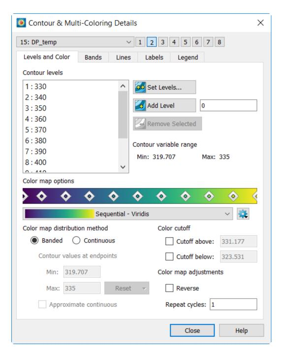
You'll notice after changing the Parcel color that two contour legends appear on screen. This is because the parcels are colored by DP\_temp while the slice is contoured by temp. Since both contours are in reference to temperature, we can update the contour levels of both contour groups.
