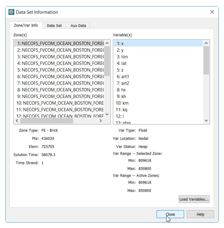
In the Zones field, we can see that the NetCDF ocean model has loaded 24 zones. In this case, each zone represents a new timestep of the data so we have 24 timesteps in total. We can also see in the other column the variables that have been loaded from the dataset. Close the Data Set Info dialog for now.
