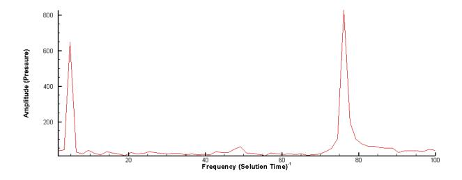
Looking at this plot, we can easily see that there is a low-frequency spike at around 5 Hz and a higher-frequency spike at about 77 Hz. This matches what we see in the time series plot: a lower-frequency (high-period) wave overlaid by a higher-frequency (low-period) wave. The combination makes the time series plot look a little jagged.
