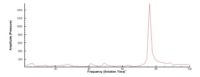
Here, the main frequency is the one we previously saw at around 77 Hz. The lower frequency around 5 Hz is no longer there, indicating that we are probing far enough away to avoid the effects of the turbine blades. We can conclude that the 77 Hz frequency is an input boundary condition.
