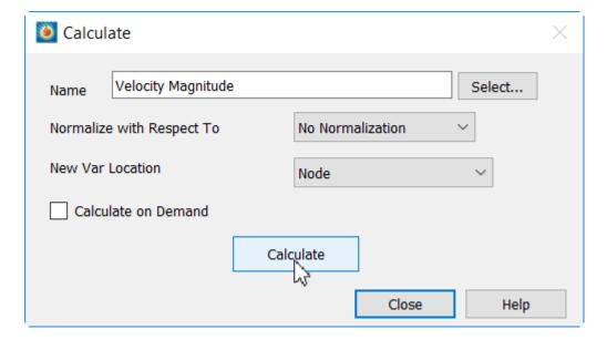
Then select Calculate and the Velocity Magnitude variable will begin the calculation process for all zones. Information will appear upon completion that the calculation was successful. Now in the Data Set Info dialog (Data→Data Set Info) you can see the Velocity Magnitude variable at the end of the variable list.
