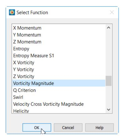
As you can see, there are literally dozens of variables that Tecplot 360 can calculate for you. Choose Vorticity Magnitude in the list then click **OK** to return to the Calculate dialog. The default options in the Calculate dialog are acceptable (note that the Calculate on Demand checkbox is checked!) so go ahead and click **Calculate**.
