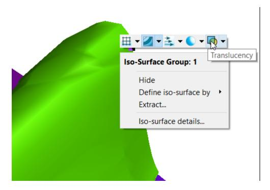
Now you can see the Mach 1.2 iso-surface inside the Mach 1 iso-surface. Rotate the plot and see! This is the shock surface where the transition between subsonic and supersonic is happening. Here's our final iso-surface plot.
