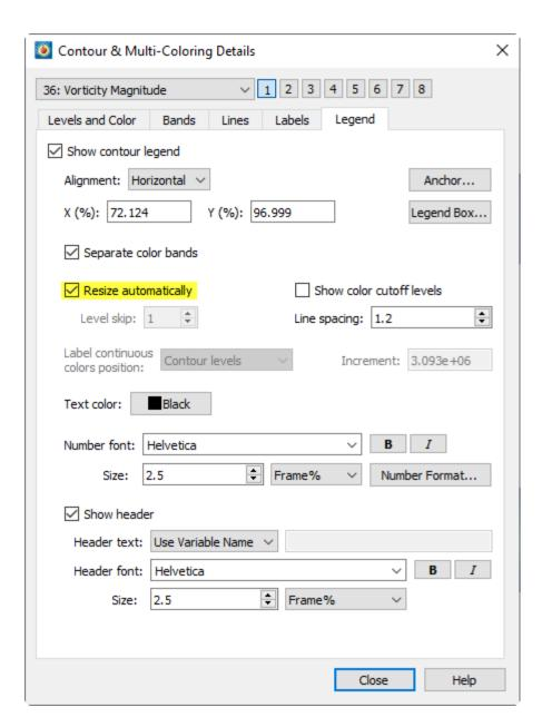
One last trip to the Contour Details dialog. Switch to the dialog's Legend page, change the alignment to horizontal, and activate the Resize Automatically checkbox.
