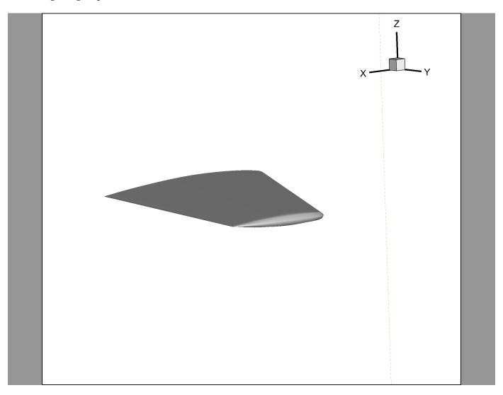
This is the bounding box of the FluidVolume zone, which represents the air around the wing. This zone does not have any style (that is, visual appearance) so it would normally be invisible. Tecplot 360 adds the dashed orange line so that you know it's there and can see its dimension.
