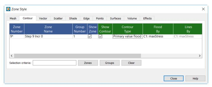
Close the **Zone Style** dialog and notice that the resulting plot contains only yellow and blue. The blue cells occur when the Von Mises stress threshold is met or being exceeded.
