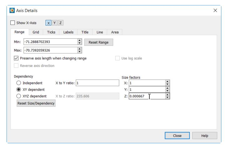
Note that the Z-axis is still exaggerated even at this ratio, but it gives a better understanding of the overall scale.
