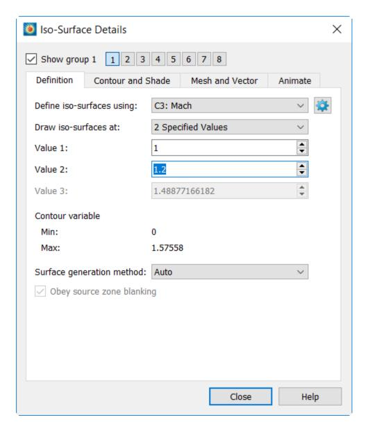
Where's the second iso-surface? Well, it's closer to the wing than the first one, so it is hidden. Let's make the iso-surfaces partly transparent so we can see the second one inside the first (and also, dimly, the wing surface inside the second).
