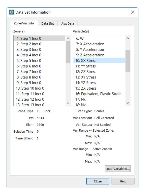
Next, select **Tools>FEA Post-Processing** to open the **FEA Post-Processing Window**. Under the **Derive Variables** section derive "**Von Mises Stress/Strain**" from "**Stress**" (the Stress variables shown below). Click **Add to Data Set**. Now on the Data Set Information page, Von Mises Stress appears as variable 33. Close the FEA Post-Processing dialog and close the **Data Set Information** dialog.
