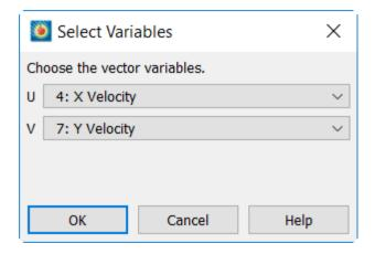
After you've accepted the vector variables, choose the streamtrace tool in the main toolbar, or in the Plot sidebar next to the Streamtraces checkbox.
