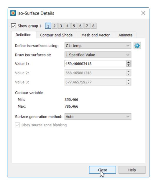
Since we want to visualize a flame front, use the variable temp set to Contour Group 1. Also select the Contour tab on the Iso-surface Details dialog and verify the Iso-surface is being contoured by temp as well.
