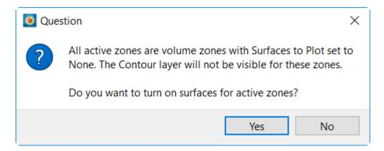
Turning on the surfaces of volume zones can be a resource-heavy operation as it requires loading the entire volume zone and calculating which cells represent the outer surface.
