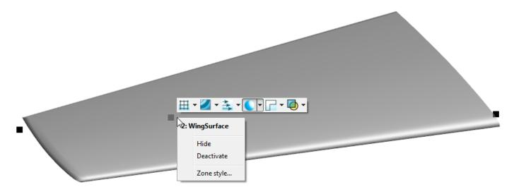
From left to right on this toolbar are buttons that allow you to turn on and off the mesh, contours, vectors, shade, edge, and translucency. Click the first button to display the mesh for the WingSurface zone, as shown here.
